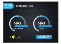
Turn the rotary knob to select your expected parameter sign. Press the rotary knob, there will appear a triangle sign, indicates the current parameter is available to set when you turn the rotary knob. Press the rotary knob again, the triangle sign disappeared indicates that the machine recover to the parameter selection state again.
