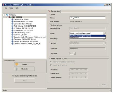
Figure 3.27 Wireless Settings: Mode Drop-down Menu
