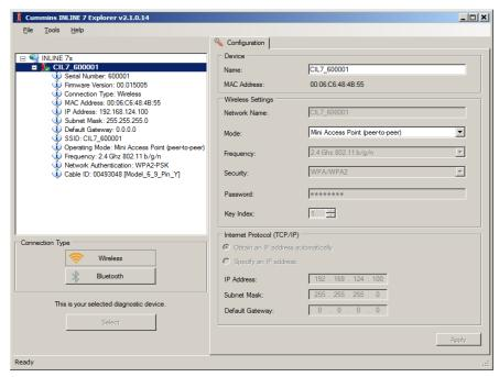
Figure 3.26 Configuration Tab
