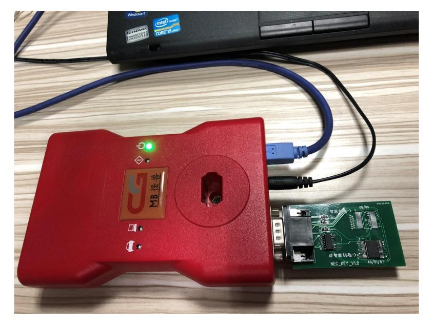
Disassemble the key, take the chip out, and solder it to the NEC adapter
