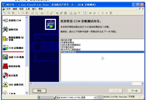
11.click "Features and Parameter" at the left column to modify engine parameters
