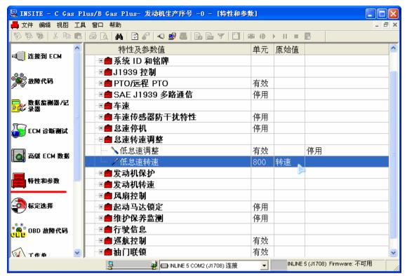
12.Click "Calibration Selection" at the left column to re-calibrate engine controller
