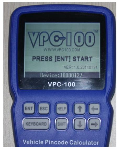
Press "ENT" button, you need to enter the machine starting password.
