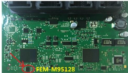
Picture 1: EEPROM position on FEM System
