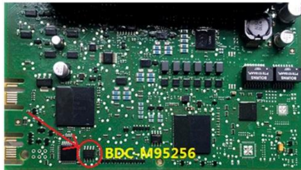
Picture 2: EEPROM position on BDC System
