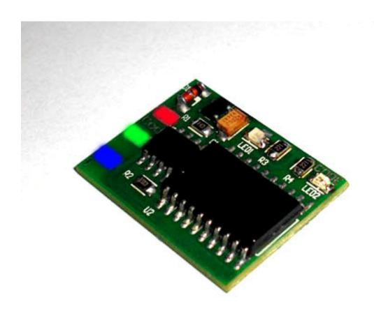
Infrared immo, pyxis 12 pin + 2 pin CAN but only occupied L (H CAN empty) LEDs green and red are flashing in the mirror.
