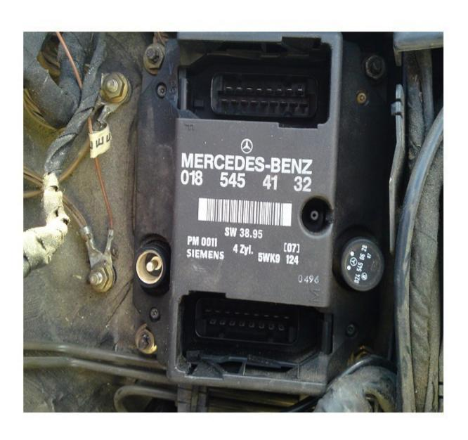
Connect emulator instead of infrared immo, pyxis 12 pin + CAN 2 pin under the feets of passenger.
