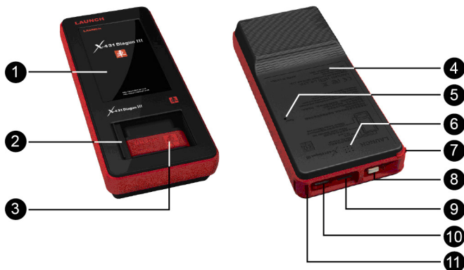
Fig. 2-2 X-431 Diagon III main unit ports and indicators
