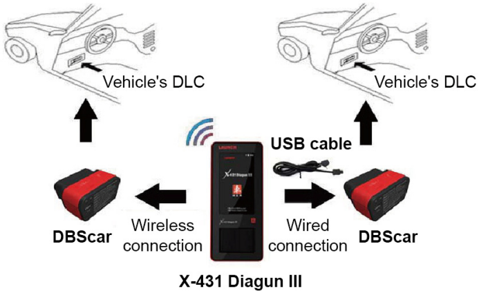
Fig. 3-2 Bluetooth (wireless) / Cable (wired) connections
