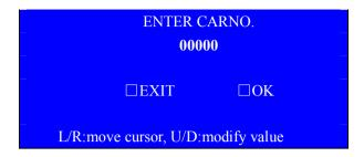
Press the keys of  $(\rightarrow)(\leftarrow)$  to move the cursor to change the digit position, press the keys of  $(\uparrow)(\downarrow)$  to change the value of some digit. When the date or the car number has been right, press the key (OK), the auto scanner will save the test results into the memory of itself.
