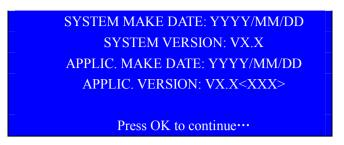
2. Press the "OK" button, then the instrument would come to the testing program. When the following display shows up, it means the connection is successful, then you may come to the next step.
