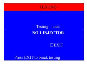
If you want to choose one actuator, press the key (OK), if the test is over, press the key (EXIT).
