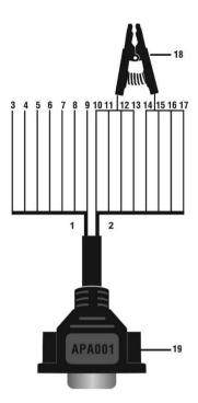
Figure 2-5 EEPROM Clamp Integrated MC9S12 Cable
