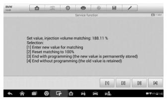
Figure 7-24 Sample Injection Rate Screen
