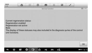
When the particle filter regeneration is complete, the tool will ask your confirmation to exit the display. Tap **Repeat** to check the status again or **End** to end the service function and exit.
