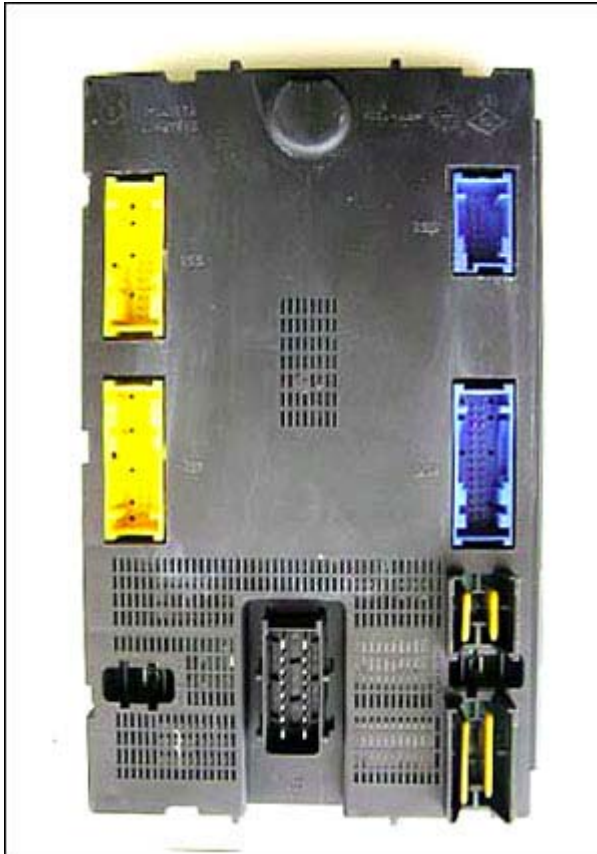
locate and read MC68HC08AZ60 Megane, Scenic UCH Siemens (in fuze box):
