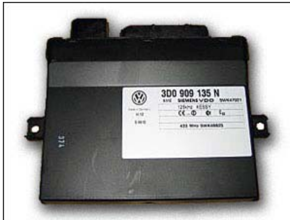
KESSY Siemens VDO (located under dashboard):
