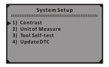
From the Main Menu: Use the UP/DOWN scroll buttons to select System Setup, and press the Y button. Follow the instructions to make adjustments and settings as described in the following setup options.
