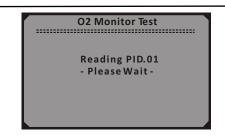
3) Use the **UP/DOWN** scroll buttons to select the O2 sensor from the **O2 Monitor Test** menu and press the **Y** button.
