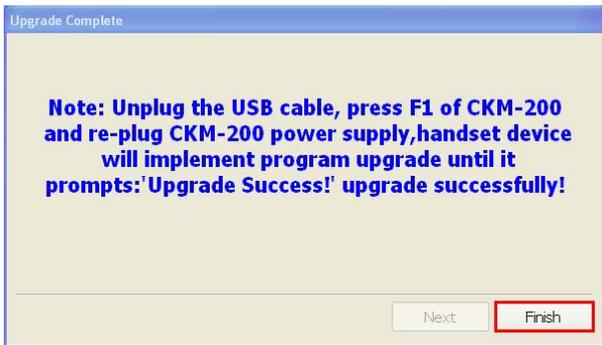
5. In the last step, it will prompt to upgrade device, you must first unplug the USB cable and device power line, press F1 of CKM-200, then plug device power line (please hold down F1 until plug the device power), handset device will upgrade procedure (in the device upgrade process, please do not off power supply) until the device prompts: "Upgrade Success!". This is a successful upgrading. As shown below:
