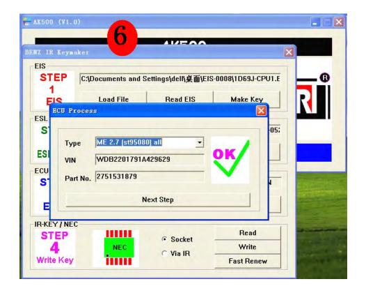
4. With "Next Step" function of the ECU to generate new data and functions with EEPROM to write back.
