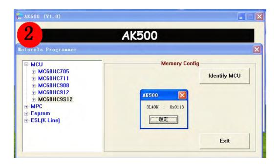
4. HC908 Series MCU: in accordance with the wiring diagram to support read and write EEPROM, a FLASH also supports reading and writing 2J74Y/4J74Y. 1J35D only allowed to deliver the ROM, can not write. (EIS's 1J35D chip can be used in place of 2J74Y or 4J74Y).
